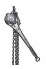
Simply by ratcheting one or two clicks per stroke in up or down mode, operator can choose quick speed of a full link or half-link rate for extra accuracy. For cramped-quarters work, ratchet handle swings to either side. This provides option of push or pull stroke to best suit conditions and preferences.
