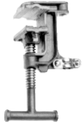
C600-2231 Bronze Body, Serrated Jaws, Bronze T-Handle, Threaded Type
