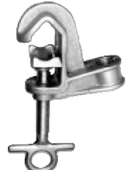
T600-0790 Bronze Body, Smooth Jaws, Bronze T-Handle/Eyescrew, Threaded Type
