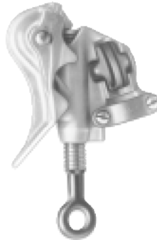
G3622-1 Aluminum Body, Smooth Jaws, Bronze Eyescrew, Pressure Type (Also Available in Threaded Type)
