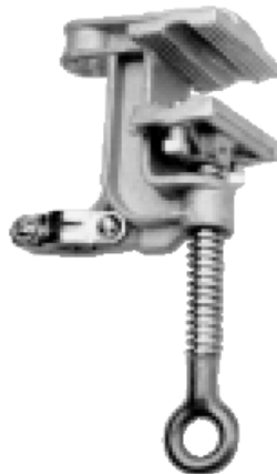
C600-2232 Bronze Body, Serrated Jaws, Bronze Eyescrew, Threaded Type
